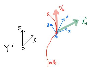
\* All the vectors are represented in the bidy-fixed coordinate Azyz (i,j,i) \* Wo is the rotating rate of the body-fixed coordinate Azyz with respect to the inertial coordinate OXYZ.
